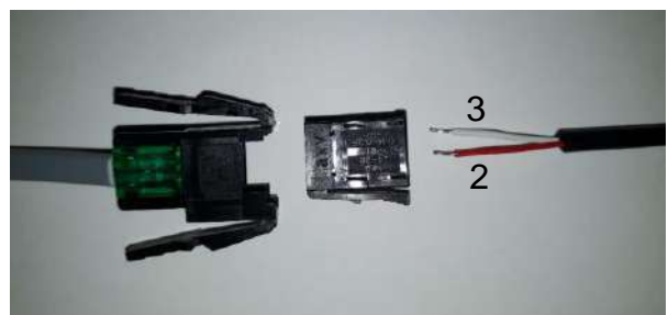
Connecting the temperature sensor cable Connect the cable to connectors 2 and 3. 1 = Remains empty 2 = Red 3 = White
